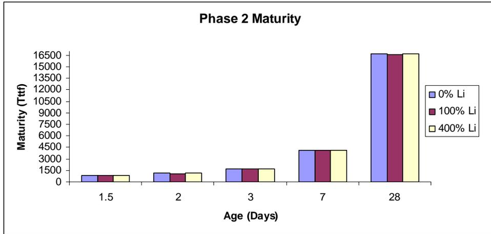
Figure 4-6. Maturity of Phase II Lab-Cured Cylinders
