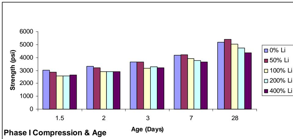
Figure 4-4. Compressive Strength of Phase I Lab-Cured Cylinders
