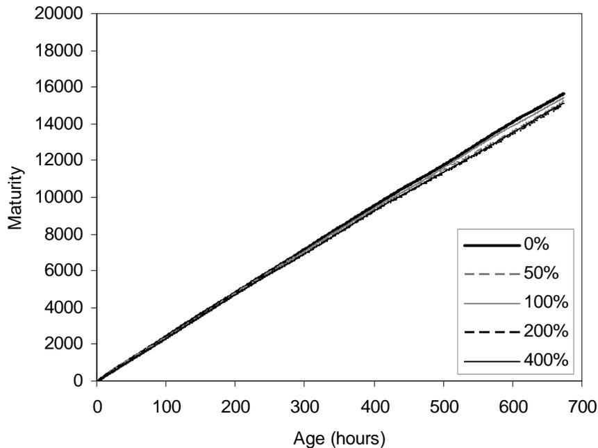
Figure 4-20. Maturity of lab specimens, Roberta cement with fly ash and Lithium
