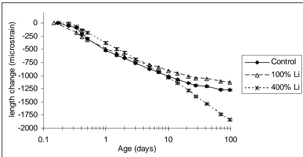
Figure 4-43. Autogenous shrinkage results for the high C<sub>3</sub>A cement
