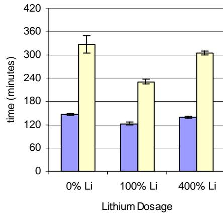
Figure 4-30. Vicat set times for moderate alkali/C<sub>3</sub>A cement.
