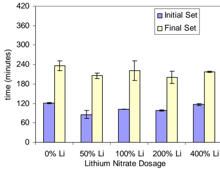
Figure 4-23. Vicat setting times for Lafarge Roberta cement, with no fly ash.
