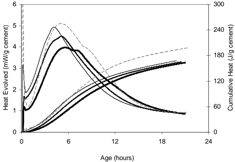
Figure 4-16. Lithium dosed low alkali cement vs. high  $C_3A$  cement
