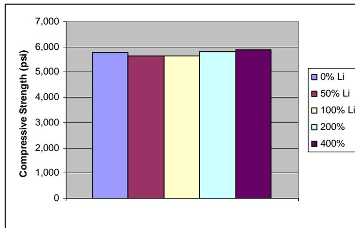
Figure 4-5. Compressive Strength of Phase I Cores
