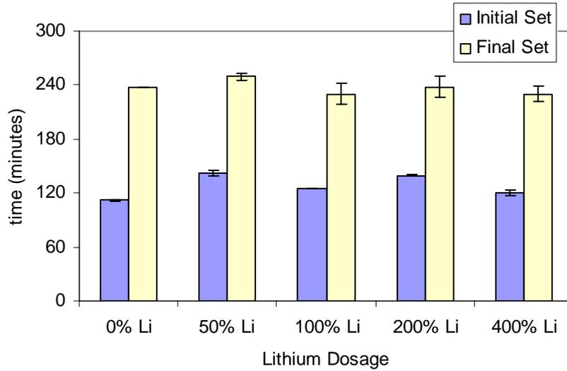
Figure 4-25. Elevated temperature set times for Lafarge Roberta cement with 20% fly ash replacement.
