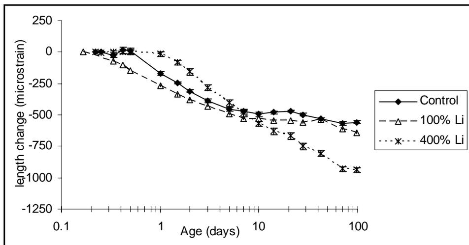
Figure 4-40. Autogenous shrinkage results for the moderate alkali/ $C_3A$  cement
