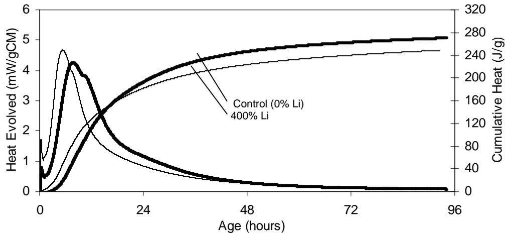
Figure 4-19. Cumulative heat curves for the low C<sub>3</sub>A cement
