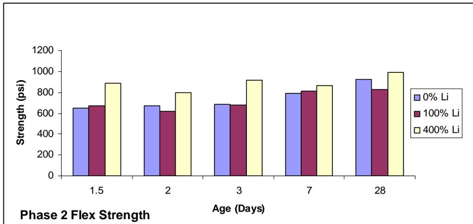
Figure 4-7. Flexural Strength of Phase II Lab-Cured Beams
