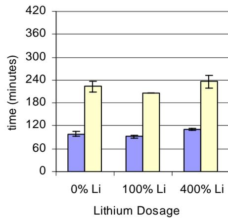
Figure 4-29. Vicat set times for High C<sub>3</sub>A cement
