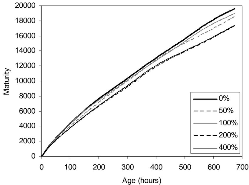
Figure 4-21. Maturity of field specimens, Roberta cement with fly ash and Lithium
