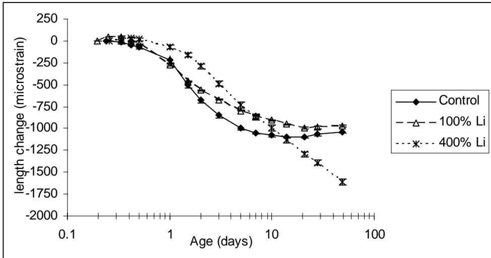
Figure 4-41. Autogenous shrinkage results for the high alkali cement
