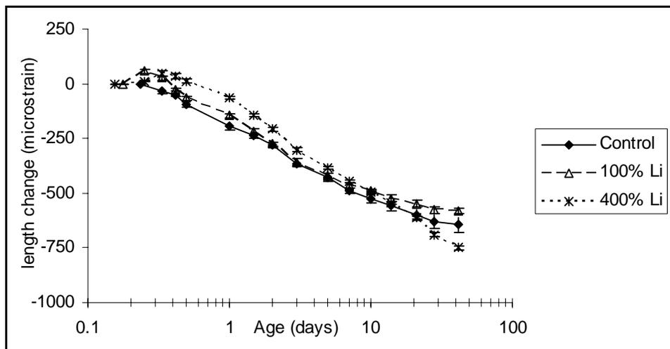
Figure 4-39. Autogenous shrinkage results for the low alkali cement
