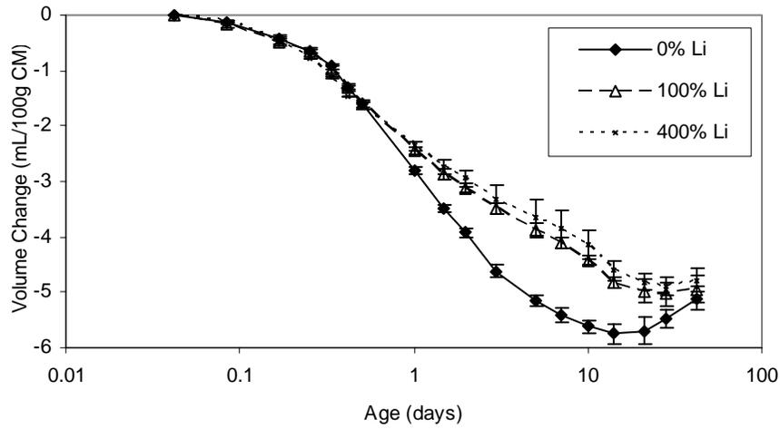
Figure 4.34. Chemical shrinkage results for low C<sub>3</sub>A cement
