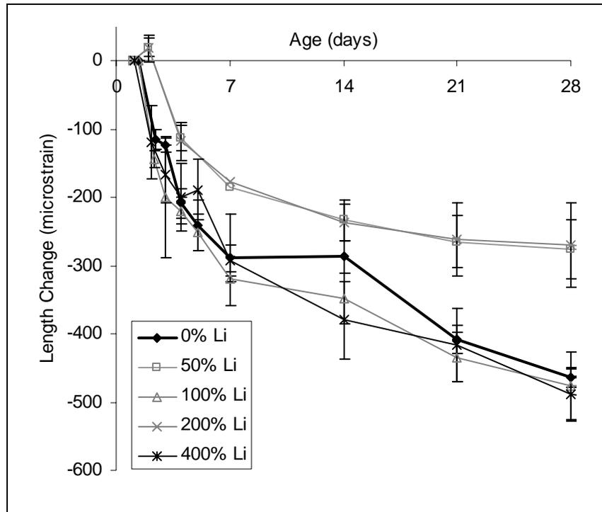
Figure 4-47. Free shrinkage results for the Lafarge Roberta cement without fly ash
