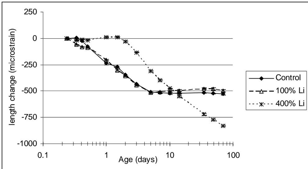
Figure 4-42. Autogenous shrinkage results for low C<sub>3</sub>A cement
