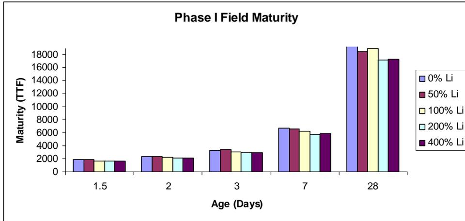
Figure 4-2. Maturity of Phase I Pavement Slabs
