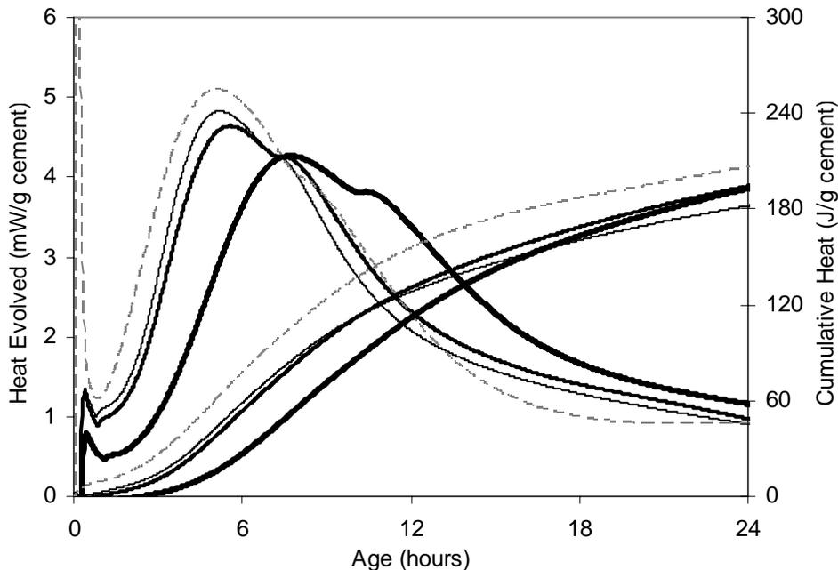
Figure 4-15. Lithium dosed low  $C_3A$  cement vs. high  $C_3A$  cement
