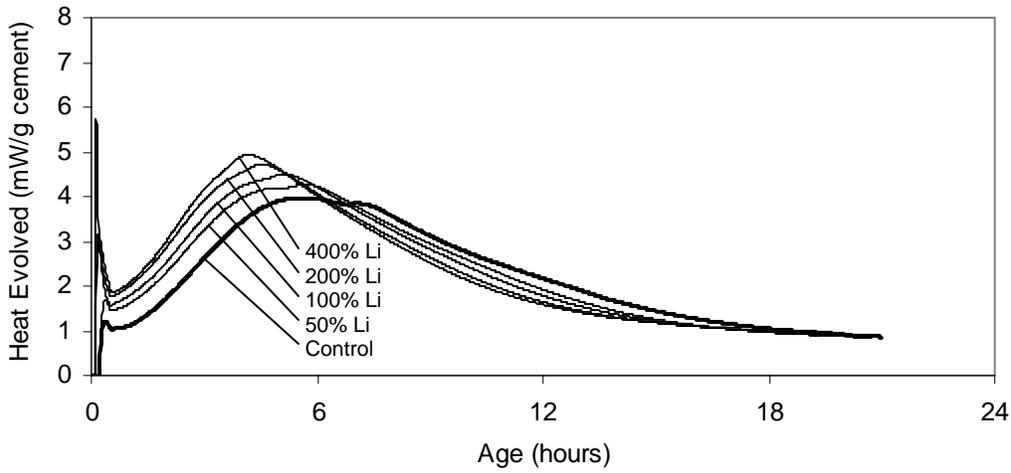
Figure 4-9. Calorimetry results for the low alkali cement
