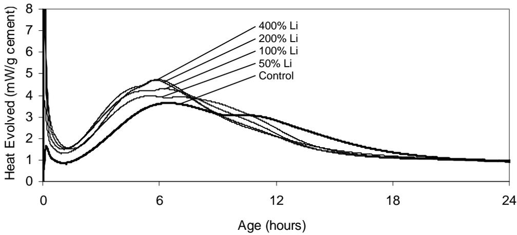
Figure 4-13. Calorimetry results for the moderate  $C_3A$  cement
