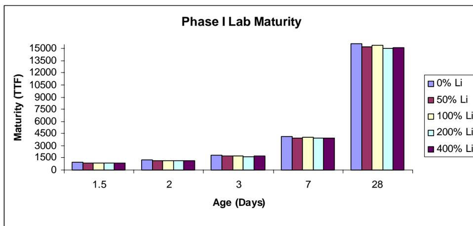
Figure 4-1. Maturity of Phase I Lab-Cured Cylinders
