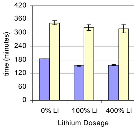
Figure 4-28. Vicat set times for Low C<sub>3</sub>A cement.
