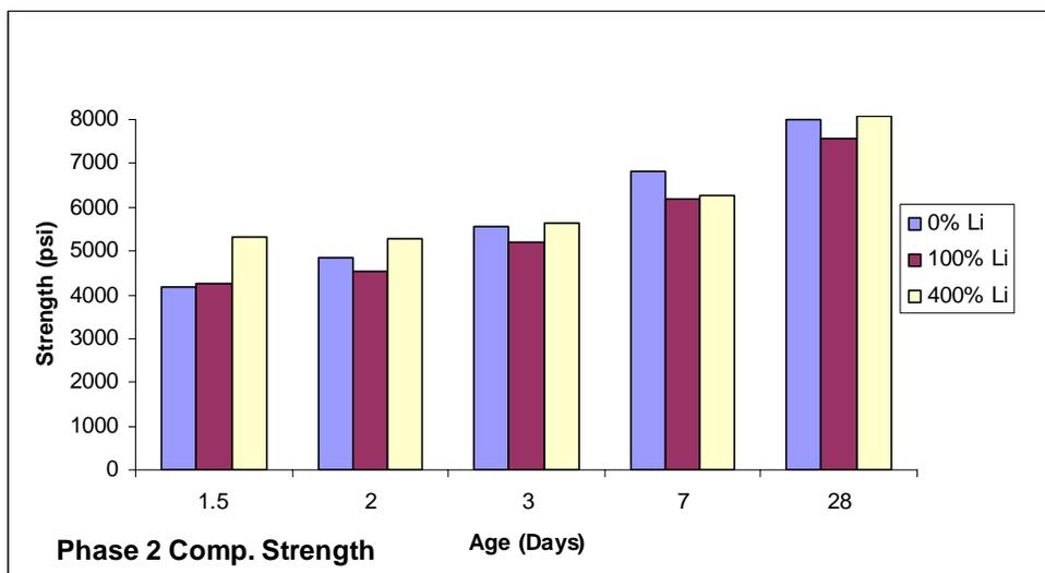
Figure 4-8. Compressive Strength of Phase II Lab-Cured Cylinders
