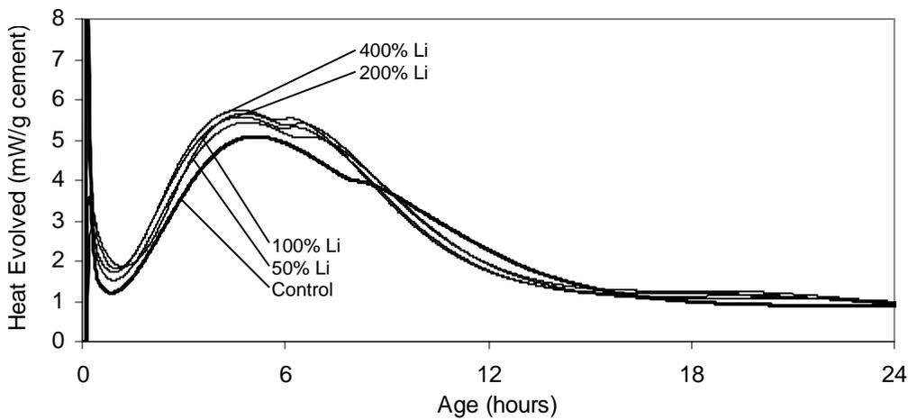
Figure 4-14: Calorimetry results for the high  $C_3A$  cement
