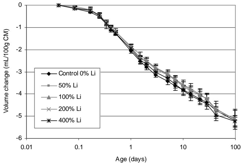
Figure 4.38. Chemical shrinkage results for Lafarge Roberta cement with 20% fly ash replacement.
