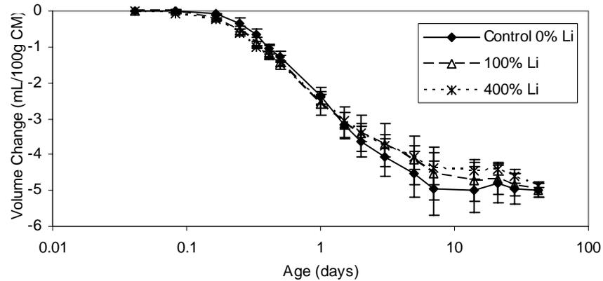
Figure 4.33. Chemical shrinkage results for high alkali cement
