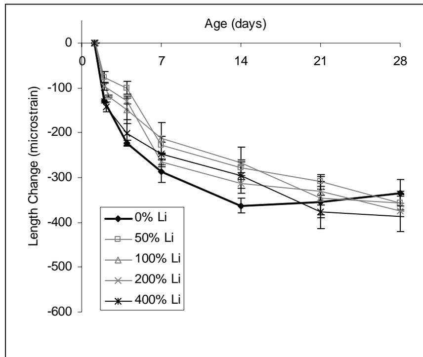
Figure 4-46. Free shrinkage results for the Lafarge Roberta cement with 20% fly ash replacement
