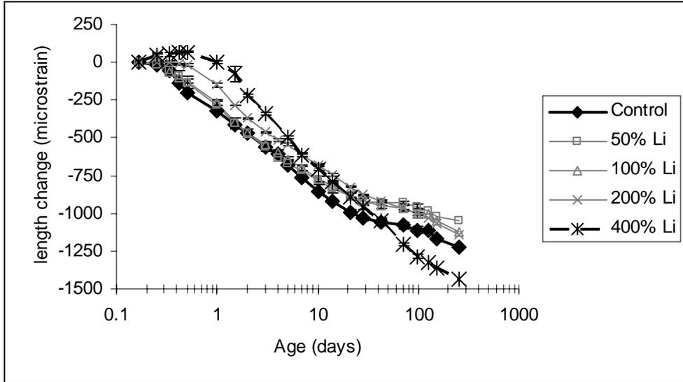
Figure 4-44. Autogenous shrinkage results for Lafarge Roberta cement with no fly ash
