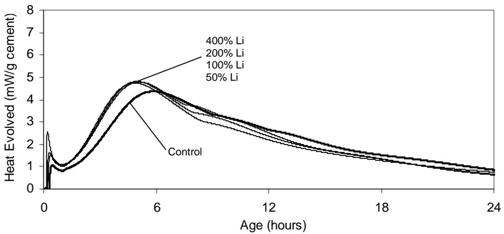
Figure 4-11. Calorimetry results for the high alkali cement
