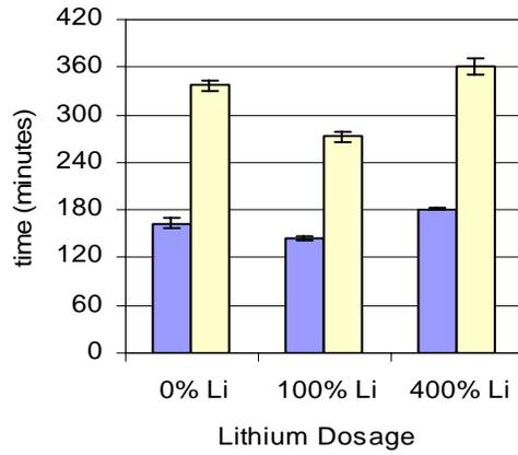
Figure 4-27. Vicat set times for high alkali cement.
