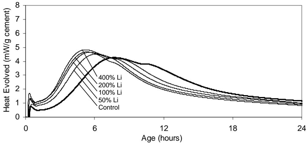
Figure 4-12. Calorimetry results for the low  $C_3A$  cement
