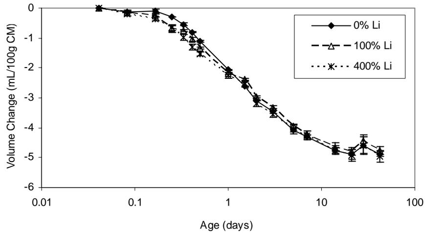
Figure 4.35. Chemical shrinkage results for moderate C<sub>3</sub>A cement
