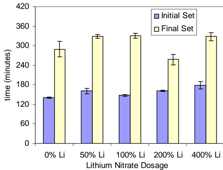
Figure 4-22. Vicat setting times for Lafarge Roberta cement with 20% fly ash replacement.
