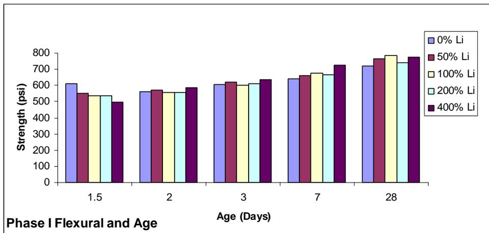
Figure 4-3. Flexural Strength of Phase I Lab-Cured Beams
