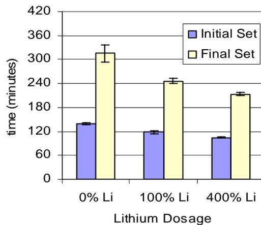
Figure 4-26. Vicat set times for low alkali cement.
