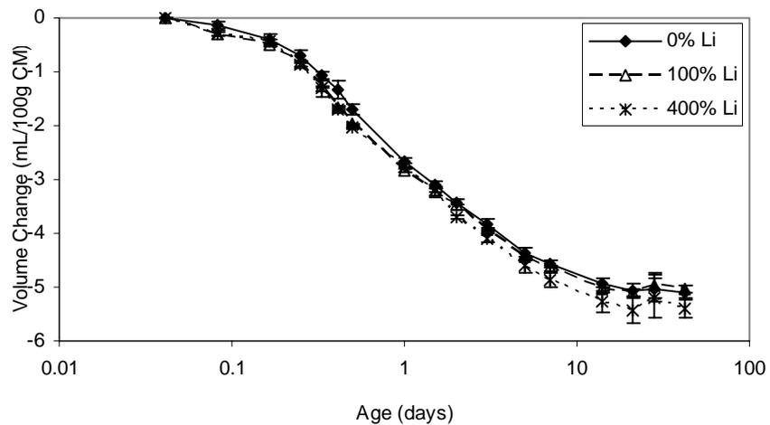
Figure 4.36. Chemical shrinkage results for high C<sub>3</sub>A cement
