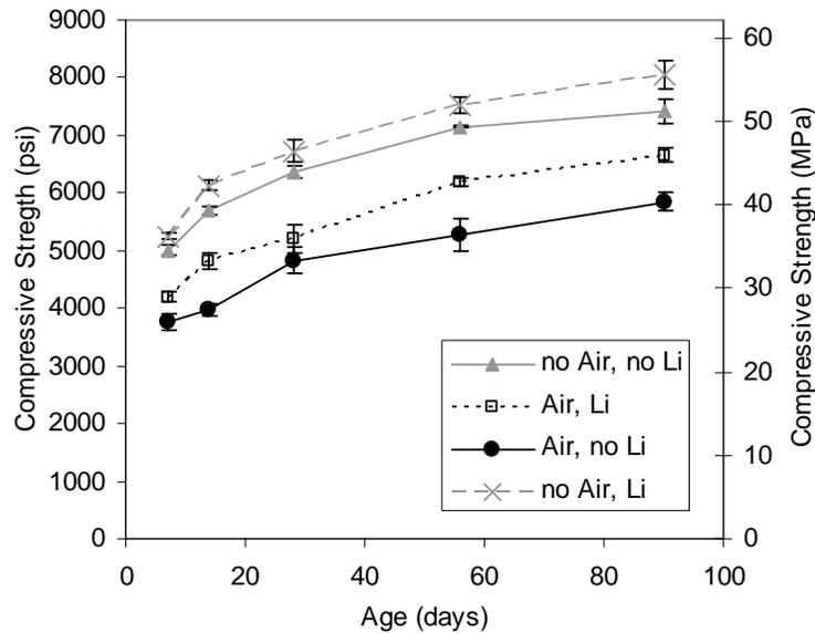
Figure 2-1. Data from McKeen et al. [2000] shows lithium-containing concrete (with and without air entrainment) to exhibit higher compressive strength, although the difference was concluded to not be statistically significant.
