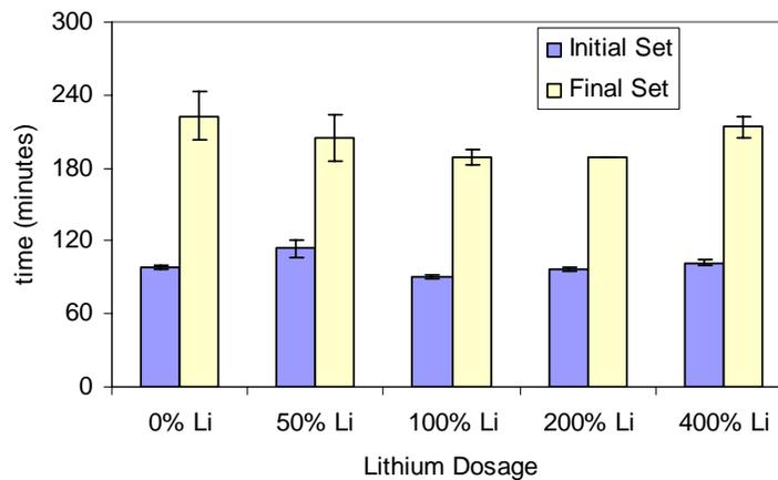
Figure 4-24. Elevated temperature set times for Lafarge Roberta cement with no fly ash.
