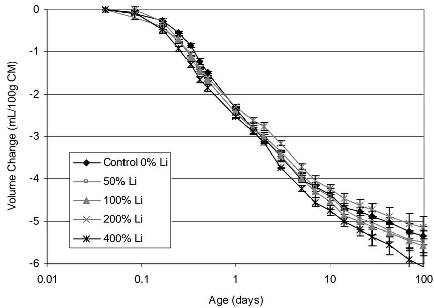
Figure 4.37. Chemical shrinkage results for Lafarge Roberta cement with no fly ash.
