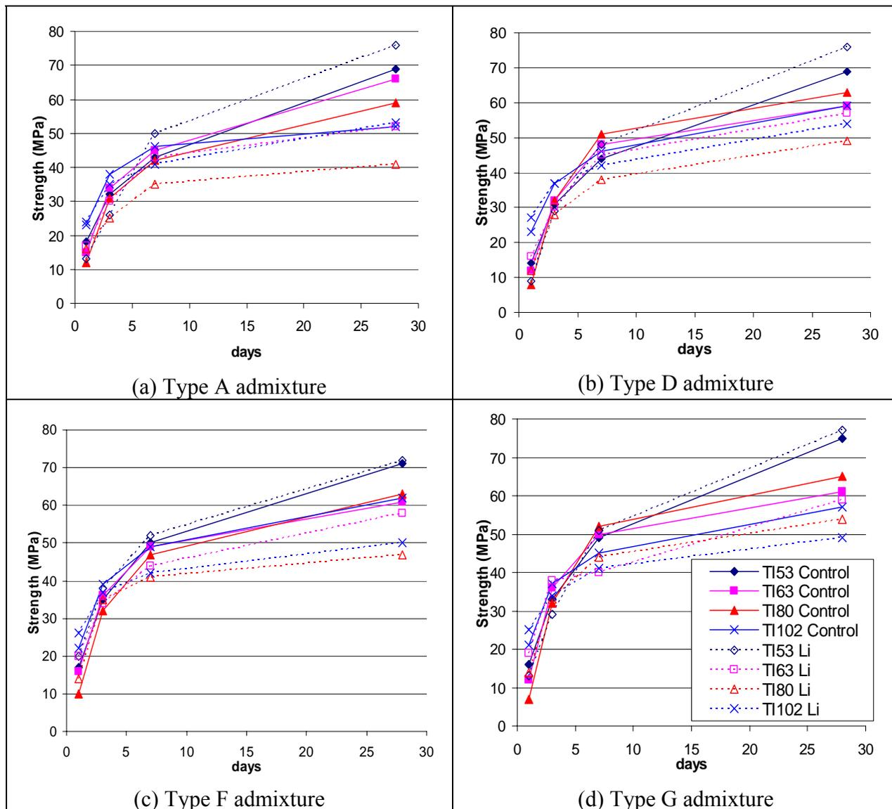
Figure 2-2. In research investigating potential interactions between LiOH admixture and ASTM Type A, D, F, and G admixtures, compressive strength was found to generally be reduced when lithium was used in mixtures with higher alkali cements. The cement alkali content is noted in the legend as the last two digits in the sample type designation (e.g., TI53 cement has a total equivalent alkali content of 0.53% and TI102 has 1.02%). Data is from Wang et al. [1996].
