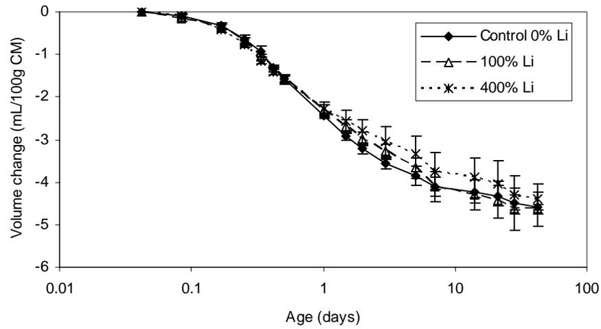
Figure 4.31. Chemical shrinkage results for low alkali cement
