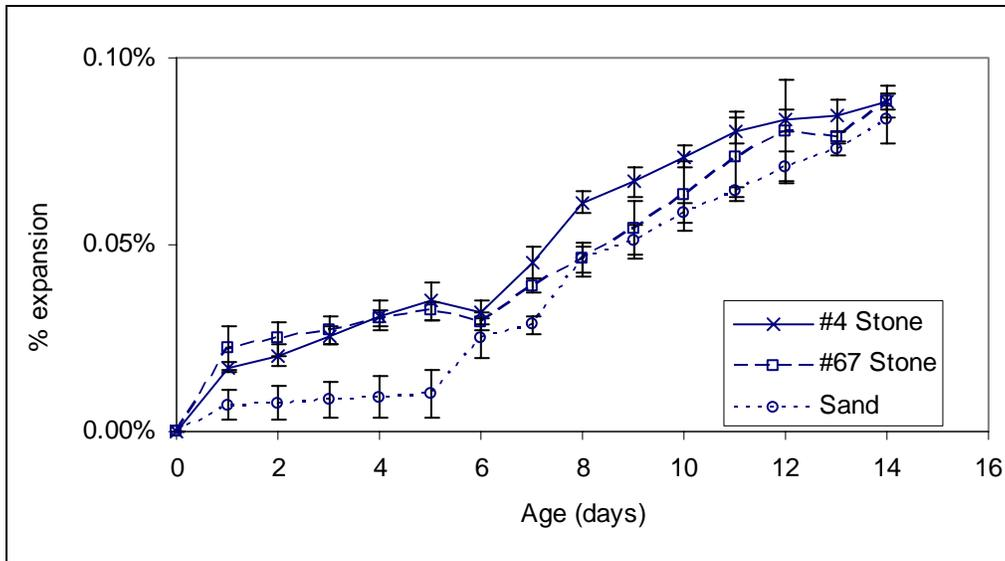
Figure 4-48. ASTM 1260 accelerated mortar-bar expansion test results
