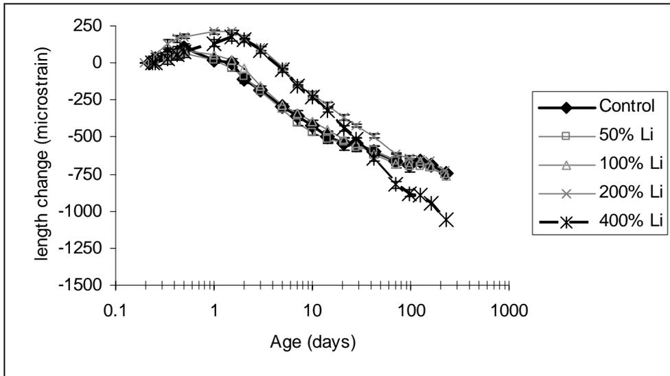
Figure 4-45. Autogenous shrinkage results for the Lafarge Roberta cement with 20% fly ash replacement
