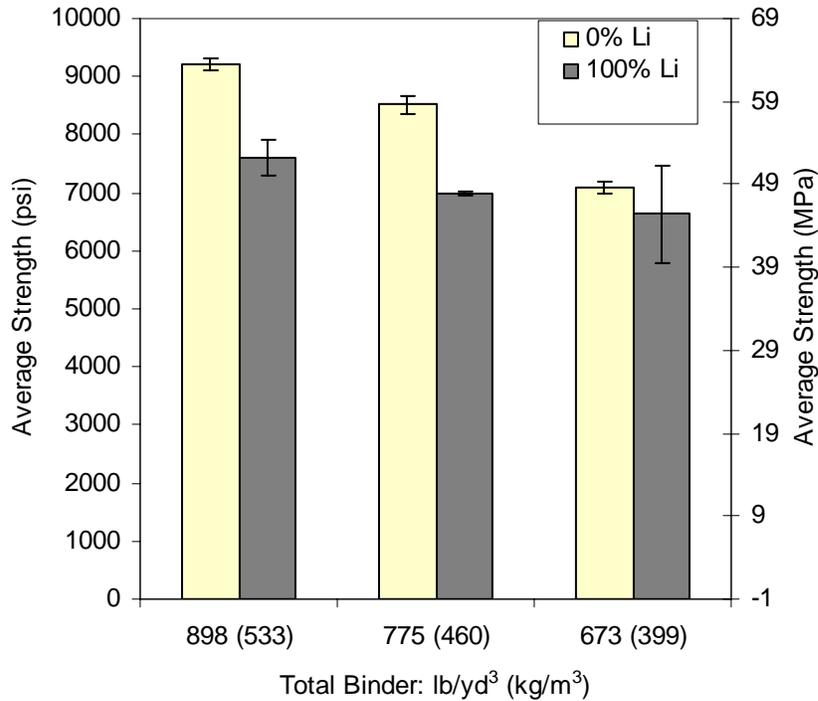
Figure 2-3. Hooper et al. [2004] report lower 28-day concrete compressive strength at 100% LiOH·H<sub>2</sub>O dosage in samples prepared and monitored by BRE.
