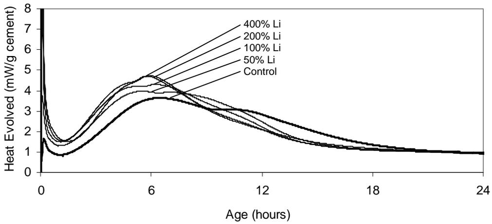
Figure 4-10. Calorimetry results for the moderate alkali cement
