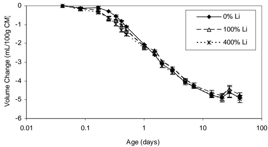
Figure 4.32. Chemical shrinkage results for moderate alkali cement
